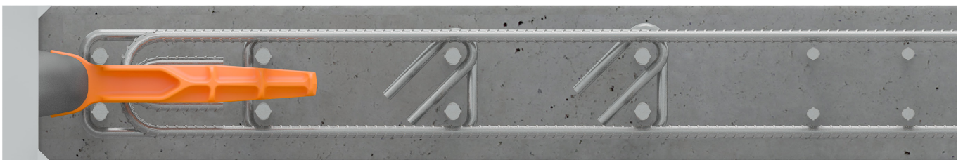
Figure 6: Double Layer Reinforcing Placement Detail
