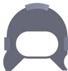
DETAIL 1.7: HPAWF Clip used to hold the hanger bar inside the anchor.
