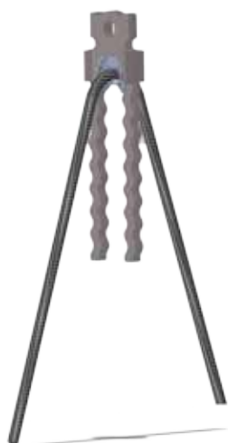
DETAIL 1.6: Cut and bend length for hanger bars installed into the anchor
