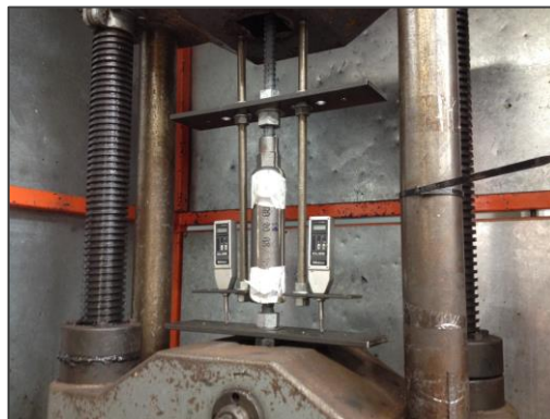
Figure 3. Tensile testing of Grout Sleeves – MoF ductile yielding
