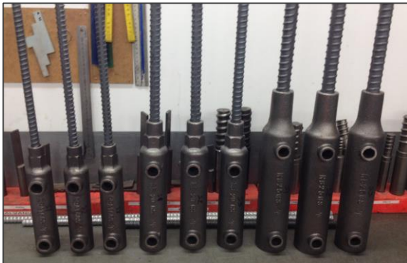
Figure 1. Sample preparation for Grout Sleeves – ReidBar™ to thread connection
