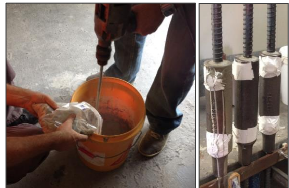
Figure 2. Sample preparation for Grout Sleeves – ReidBar™ to grout connection
