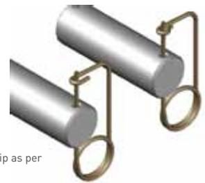
FIG 2: Secure the safety clip as per the diagram.
