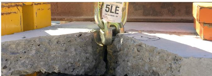
**Figure 3:** Foot Anchor tested close to an edge.
