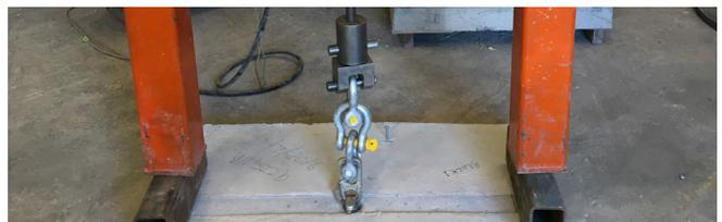
**Figure 4:** Foot Anchor tested in tension.
