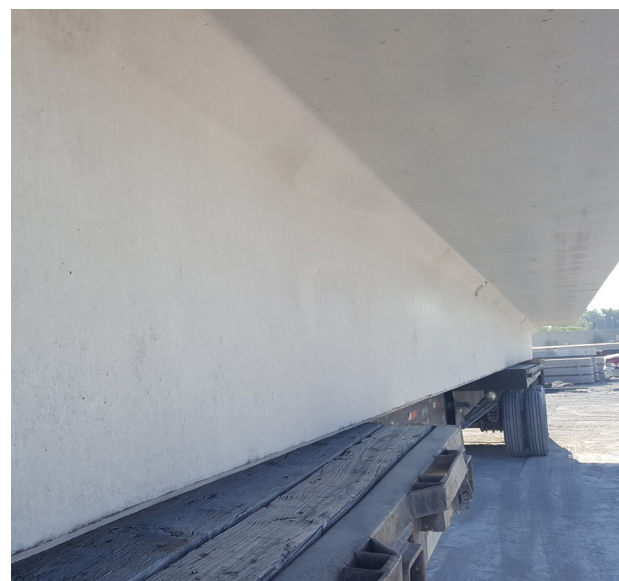
Release Agent #10 used with optimum spray application
