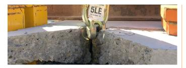
Figure 3: Foot Anchor tested close to an edge.
