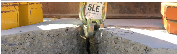
Figure 3: Foot Anchor tested close to an edge.
