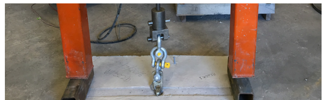
Figure 4: Foot Anchor tested in tension.
